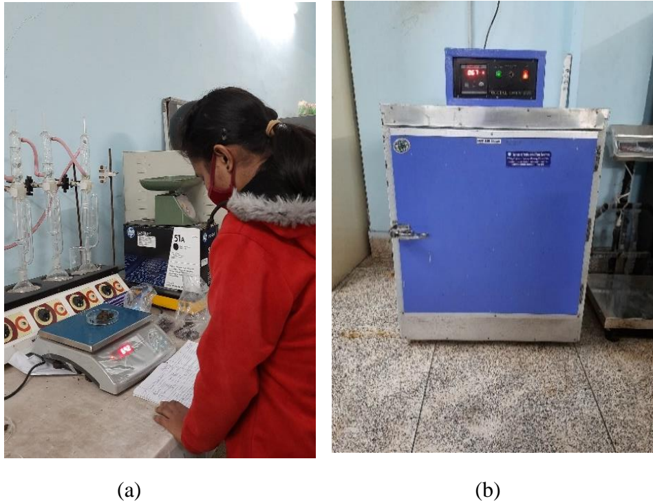
Fig. 3.9: Measurement of moisture content by oven dry method
