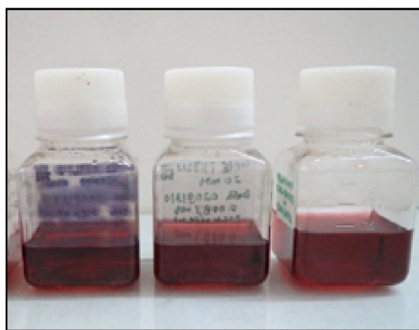
Fig. 3b : Color variation of different concentration of GNP i.e from left 20 mM, 15 mM and 10mM, respectively
