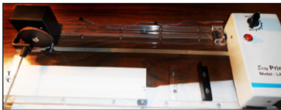
Fig. 4b : Spotting of VP7 and protein G on the strip by easy printer
