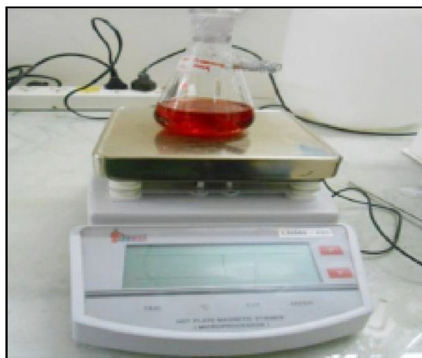
Fig. 3a : Synthesis of gold nanoparticles by citrate reduction method on magnetic stirrer with hotplate
