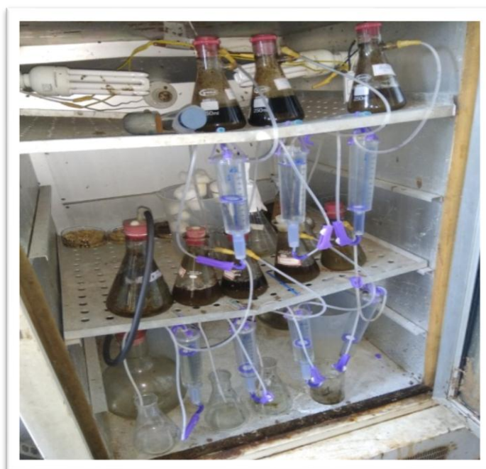
Fig. 3.4 Anaerobic digester setup for determination of biogas production potential through BMP test
