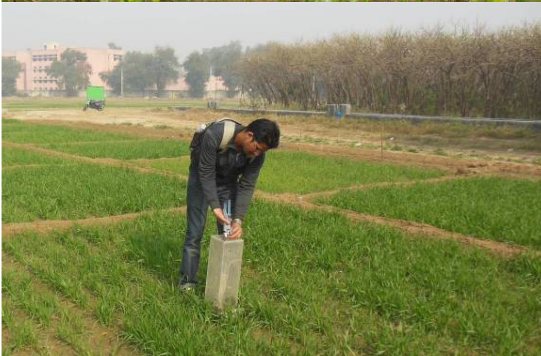
Plate 3.4 Collection of gas samples by close chamber technique
