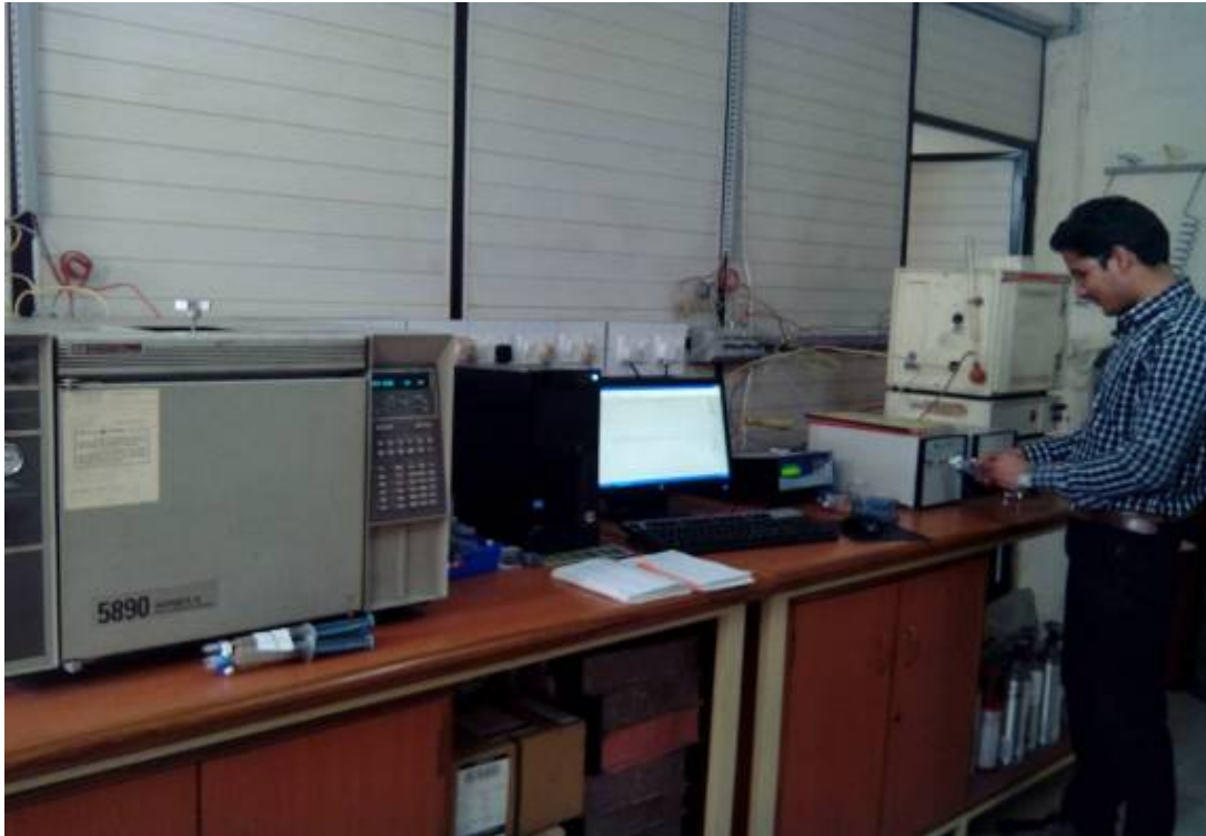
Plate 3.5 Estimation of GHGs concentration in the gas samples collected from the field by gas chromatography.
