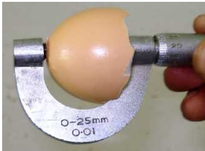
Fig. 23: Shell thickness being measured by screw gauge
