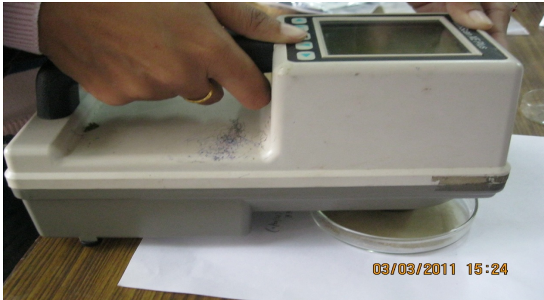
Fig. 3.7: Colour measurement using Miniscan XE plus Hunter Lab Colorimeter
