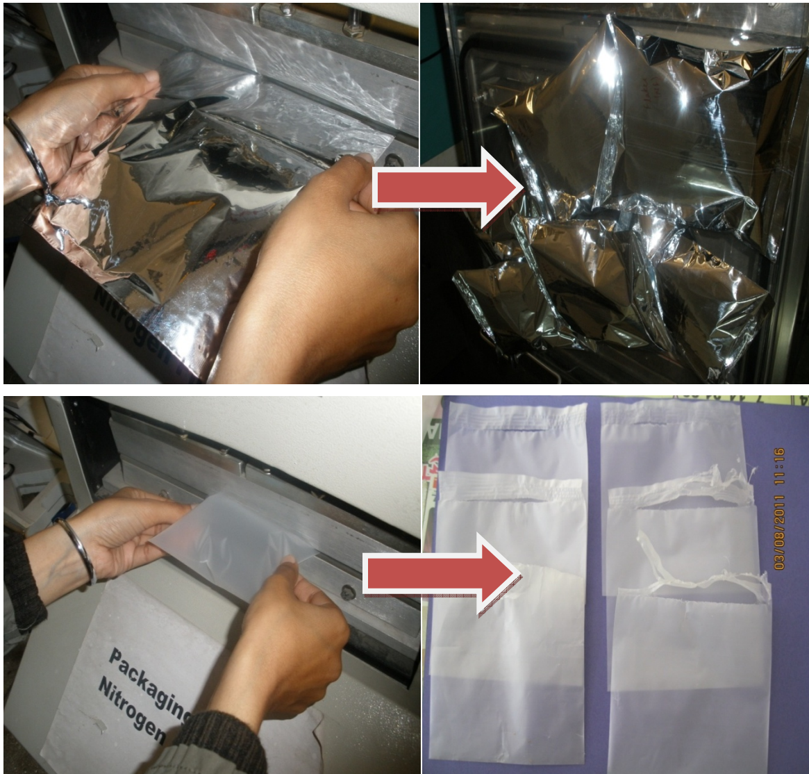
Fig. 3.5 Nitrogen flushing being done in laminated aluminium films and HDPE
