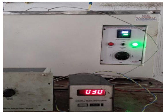
(b) Calibration in water bath
