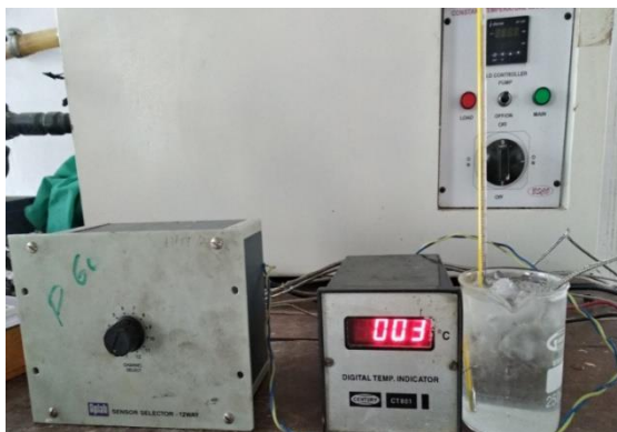
(a) Cold temperature calibration
