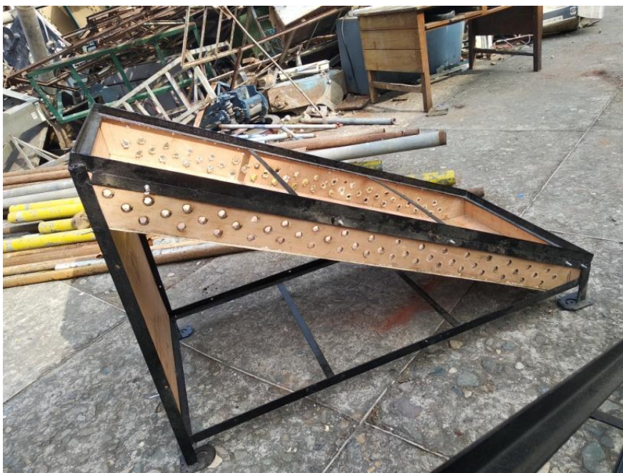
Fig. 3.9 Fabrication of cooling duct
