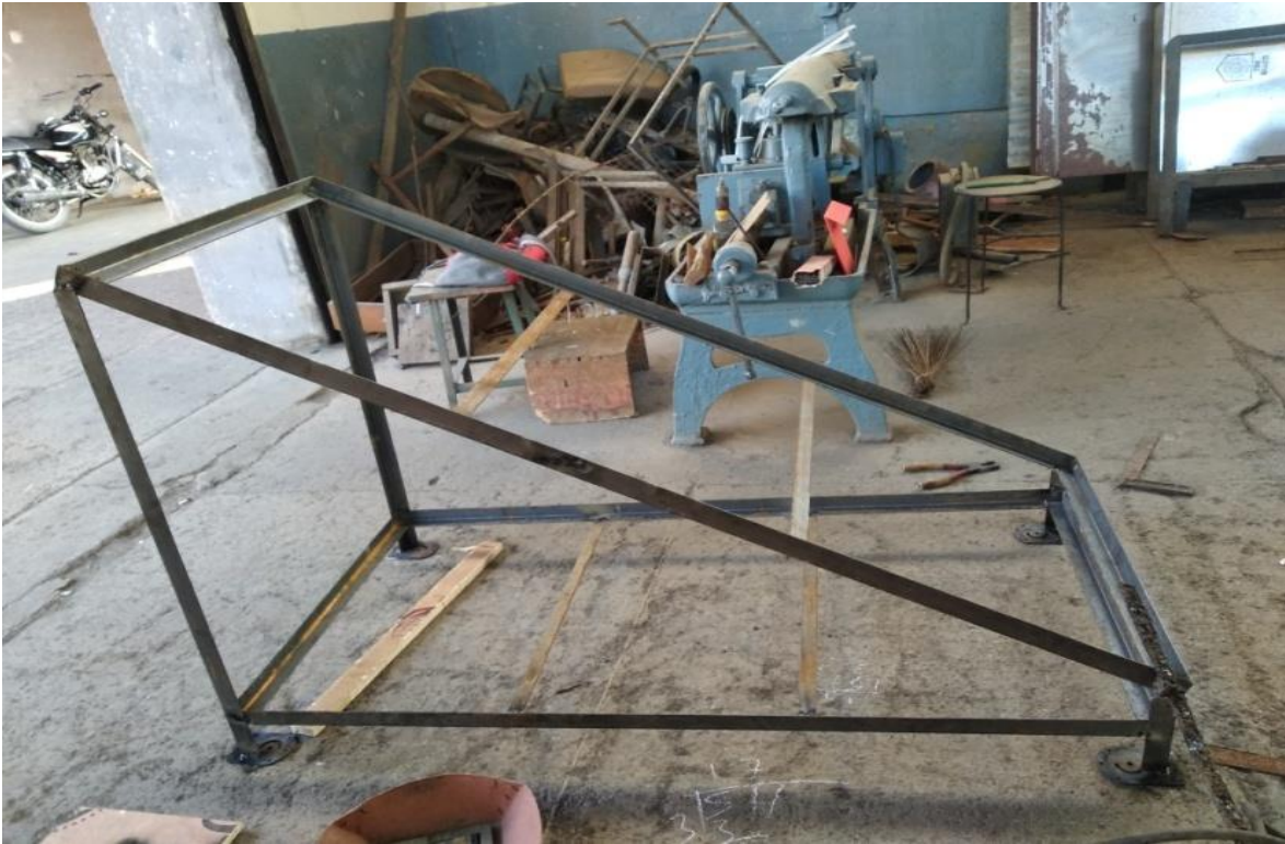
Fig. 3.2 Photographic image of solar panel stand
