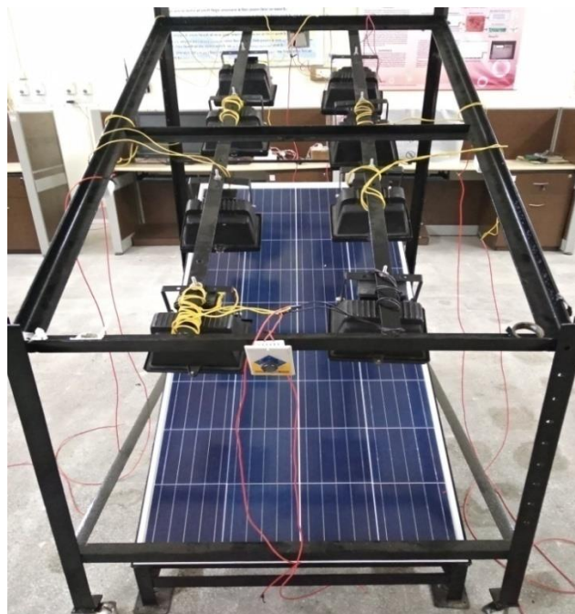
Fig. 3.8 Arrangement of halogen reflectors on solar simulator stand
