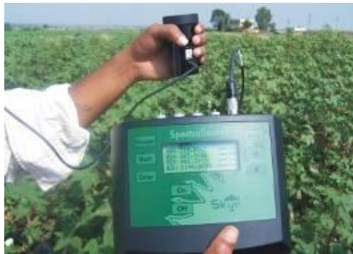
Recording spectral reflectance with a SKL 904 spectrosens-2, 4 channel display spectroradiometer
