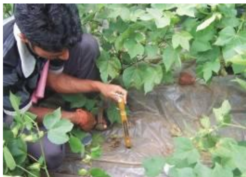
Thermometer installation In polyethylene mulched soil
