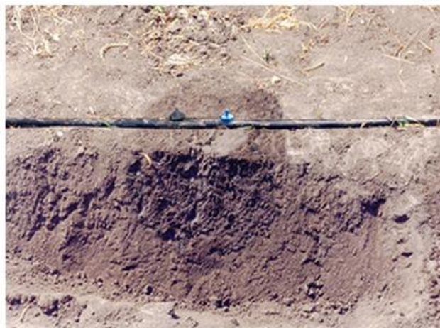
Plate 12. Diameter and depth of wetting (12 LPH dripper)
