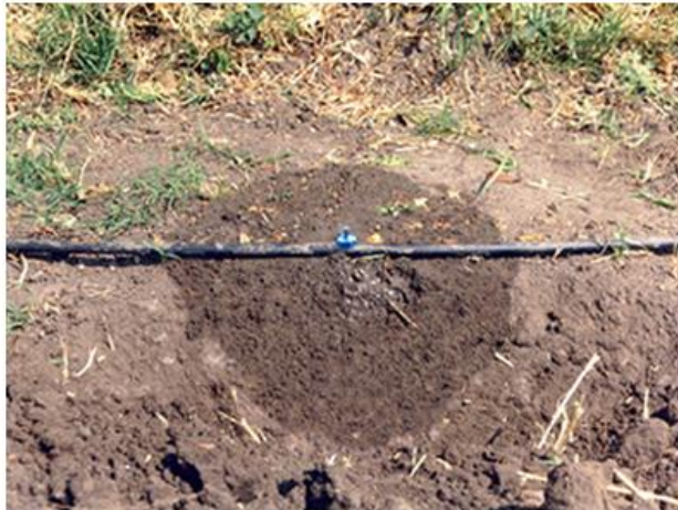
Plate 11. Diameter and depth of wetting (8 LPH dripper)
