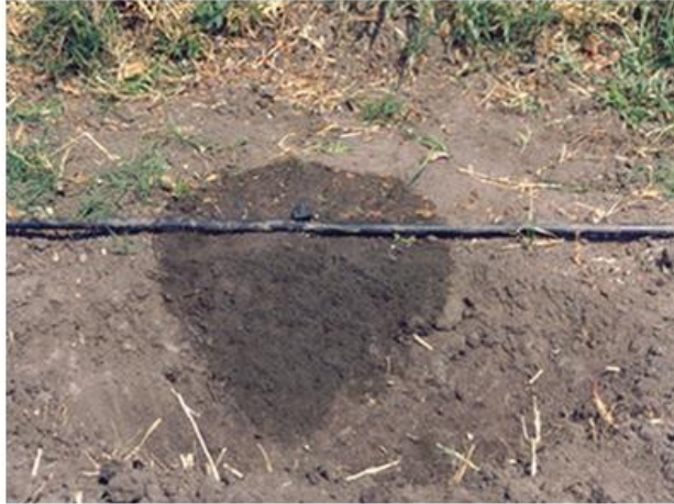
Plate 11. Diameter and depth of wetting (8 LPH dripper)
