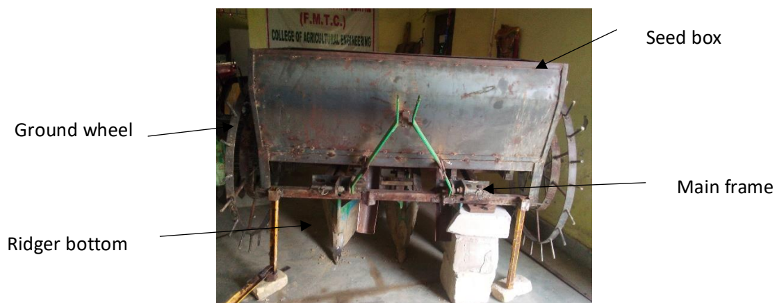
Fig 3.15: Developed turmeric planter
