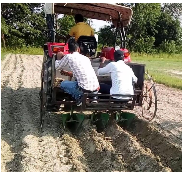
Fig. 3.17: Field testing of turmeric planter
