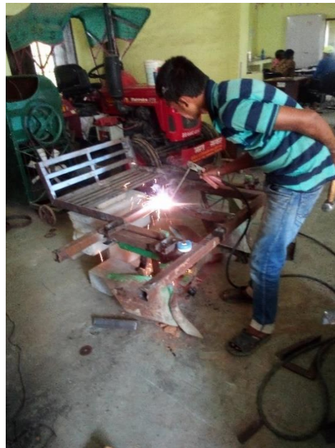
Fig. 3.14: Fabrication of turmeric planter
