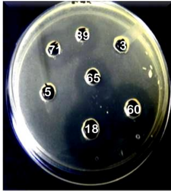
Plate 4.12. Screening of bacteriocinogenic Lactobacillus gasseri isolates using E.faecalis NCDC 114 as indicator by agar well assay
