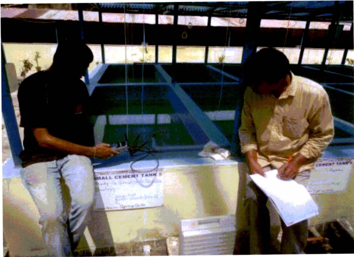
Plate 11: Measurement of DO during the experiment by “WTWOxi3205”
