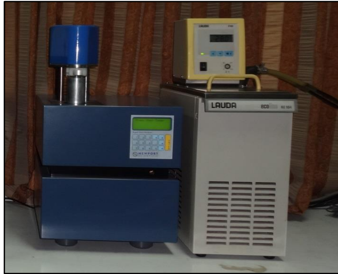
Fig. MM10. Rapid Visco Amylograph (RVA-4) measurement system with waterbath
