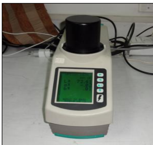
Fig. MM9. Hunter Colorflex 45/0 measurement system
