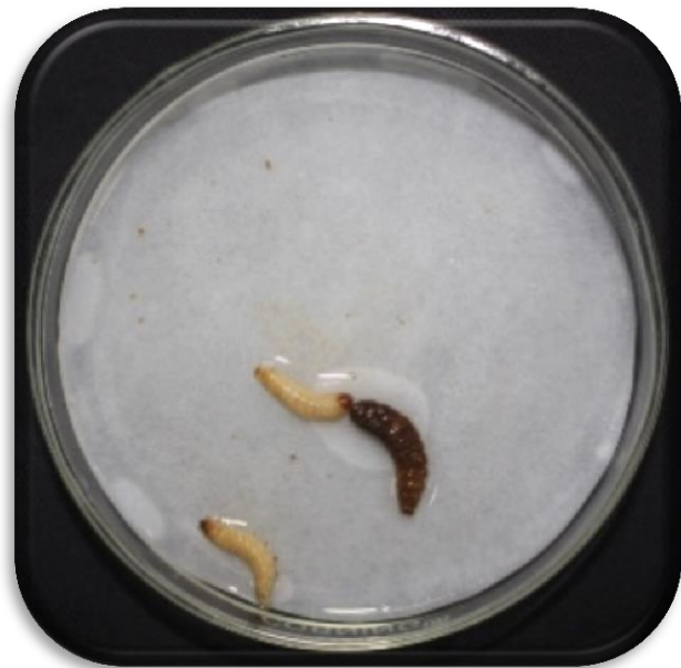
Plate 5: White's trap for in vivo mass multiplication of EPNs
