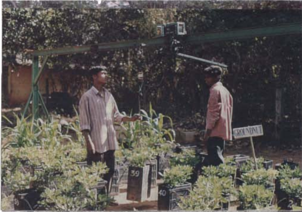
Plate-2. Foot operated peddle to lift the pots clear off the ground using a pot weighing device
