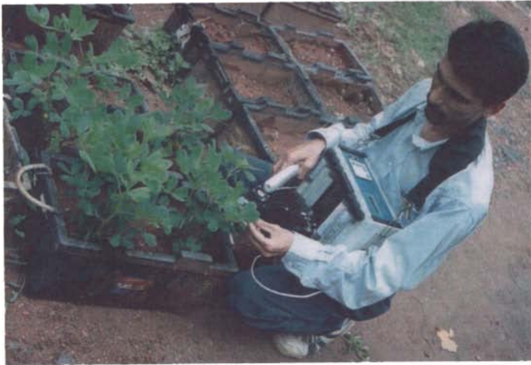
Plate-3. Recording gas exchange parameters using a portable photosynthesis system (CIRAS-1)
