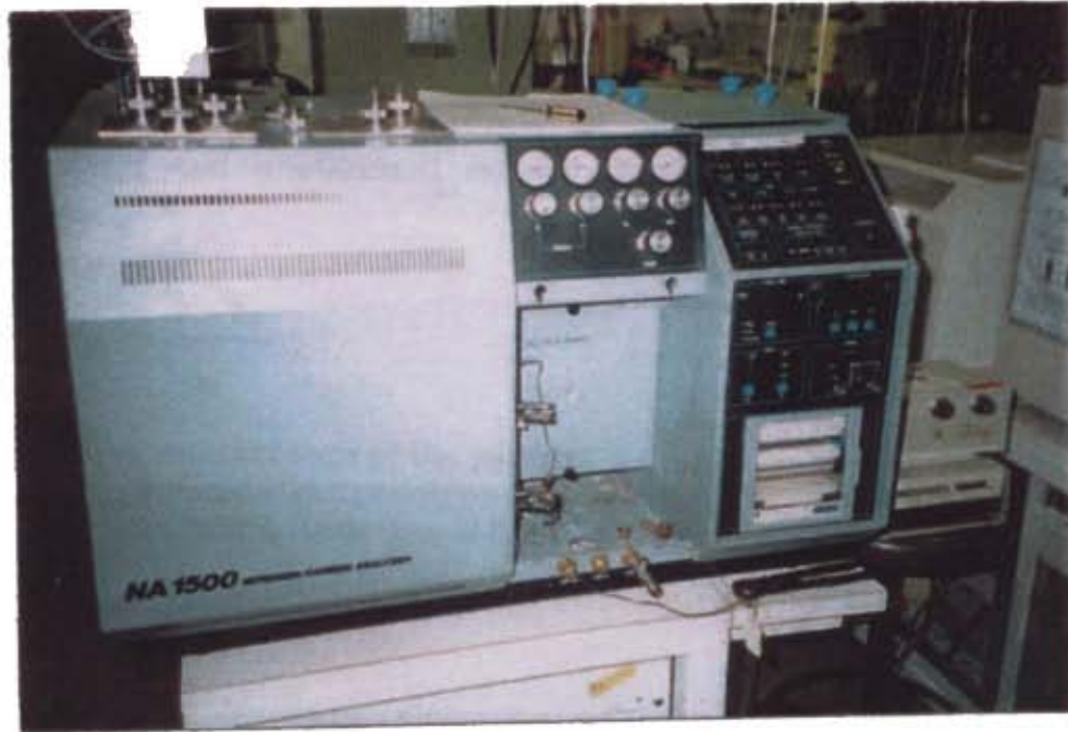
Plate-5. Isotope Ratio Mass Spectrometer (Isochrome, Micromass, UK) facility for pyrolytic determination of \Delta^{18}\text{O} in solid biomass samples at the Research School of Biological Sciences, ANU, Canberra, Australia.
