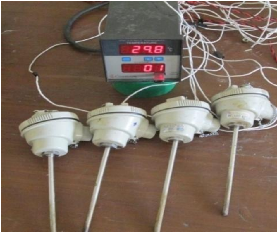
Fig. 3.12: Temperature data logger with pt 100 sensors
