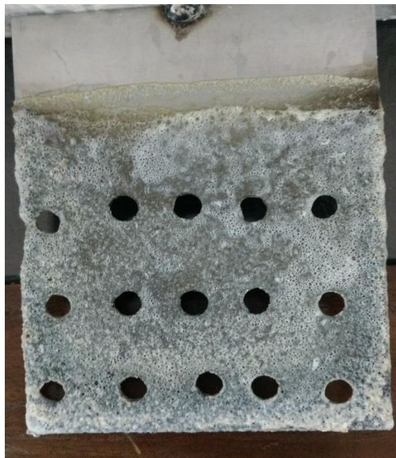
Fig. 4.18: Problem of extreme fouling in case of control in up-scaled rotating field type ohmic heating system
