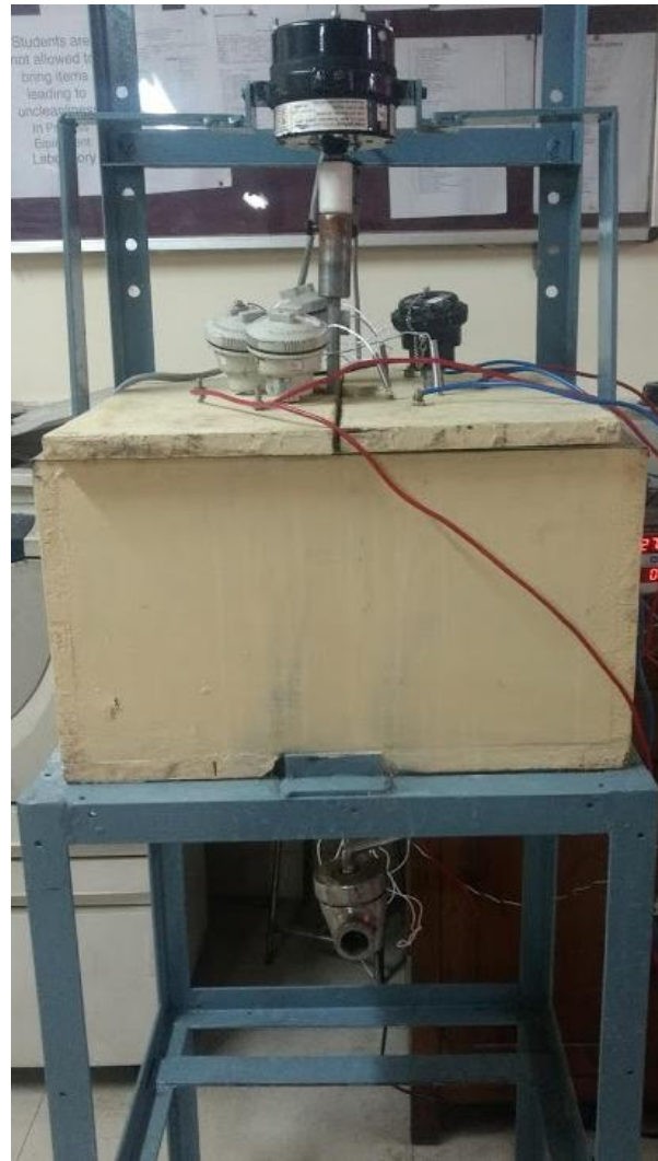
Fig. 3.3: Upscaled rotating field type ohmic heating system
