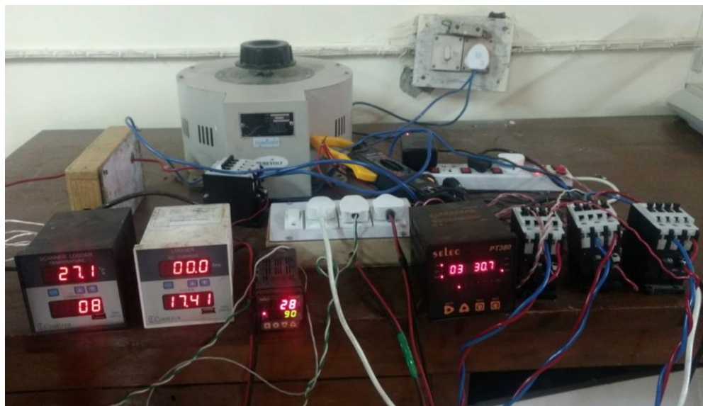
Fig. 3.4: Control system of upscaled ohmic heating setup
