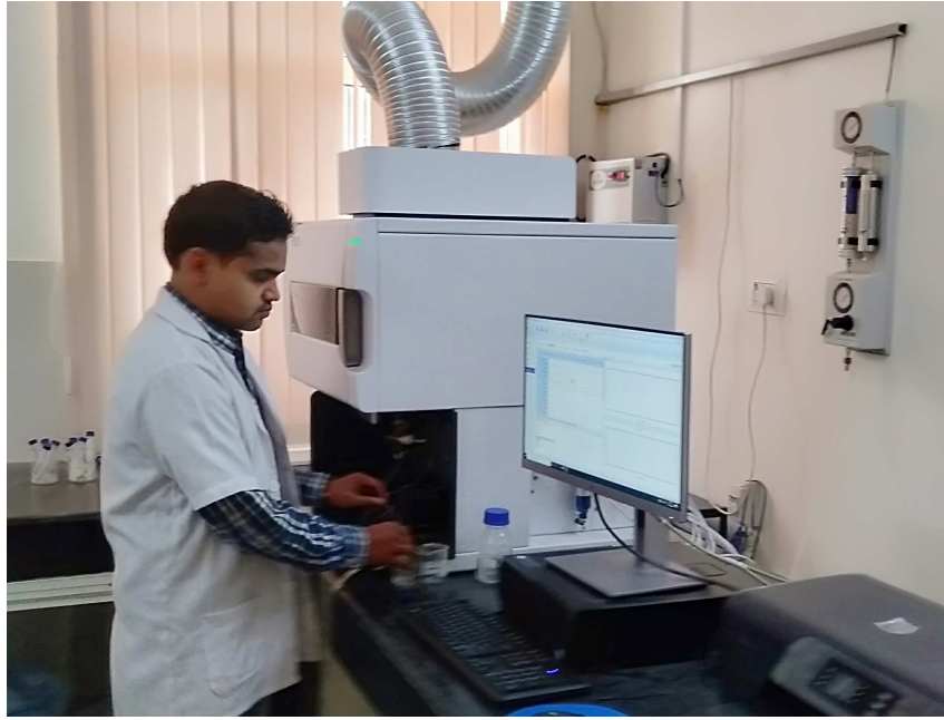
Fig. 3.23: Mineral estimation by ICP-OES
