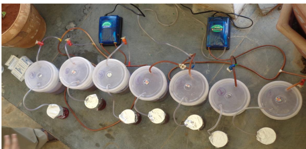
Photo 3.1: Volatilization loss experimental incubation setup
