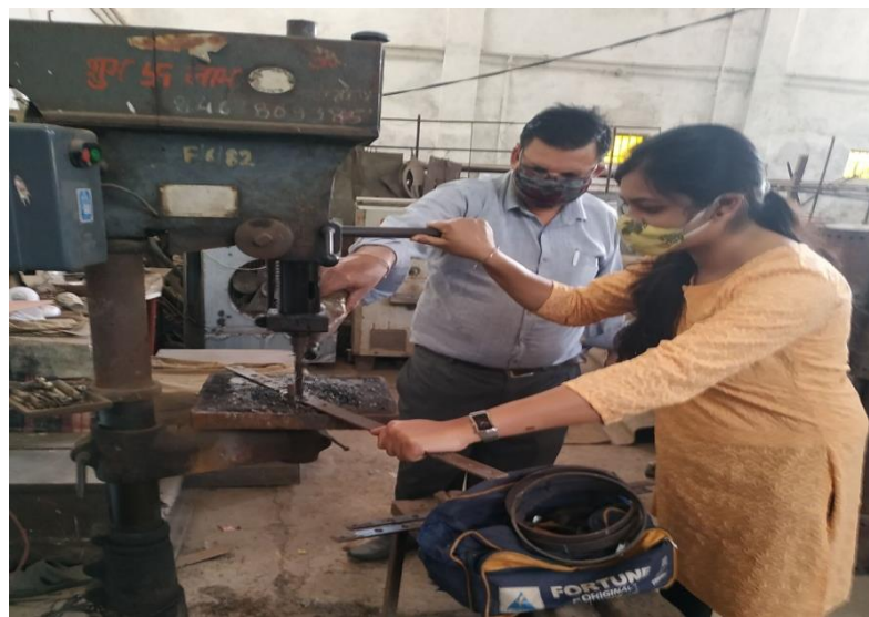
Fig.4.6: Drilling of MS plate for fabrication of crossbar
