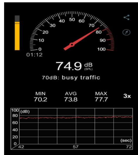
Fig 4.21 Sound testing of thresher at no load condition by mobile app (sound meter)
