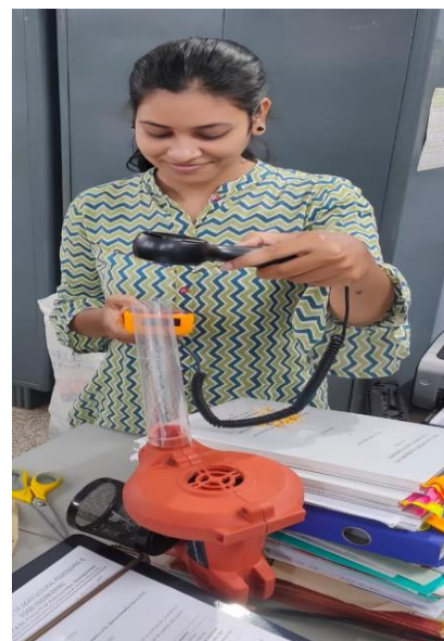
Fig 3.9 Taking reading of terminal velocity with help of anemometer
