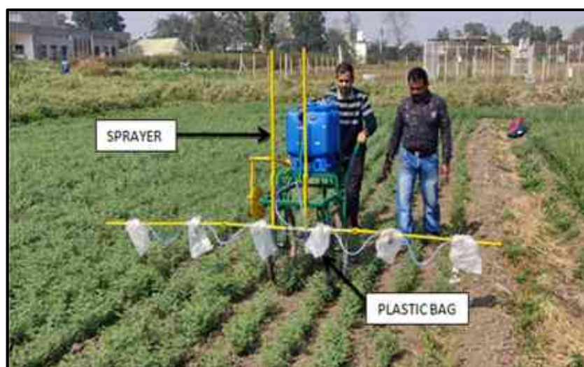
Plate 3.8 Field performance of developed sprayer
