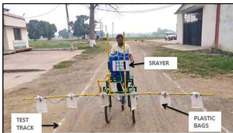
Plate 3.6 Evaluation of discharge rate in laboratory
