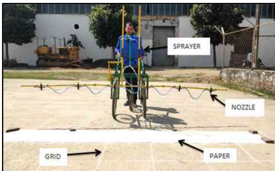
Plate 4.2 Spray overlapping test on test track
