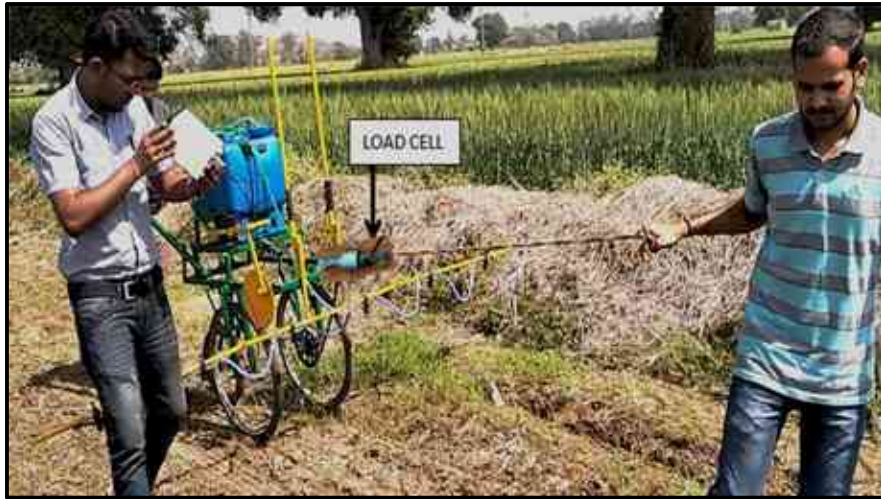
Plate 4.3 Draft measurements during field evaluation
