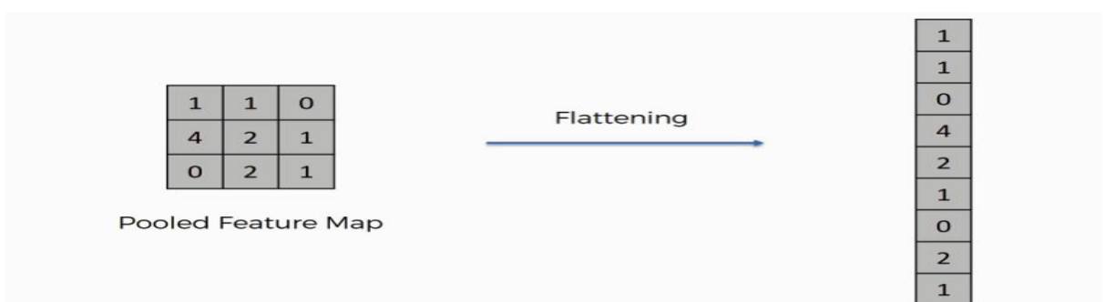
Figure 1.17: The flattening operation is depicted
