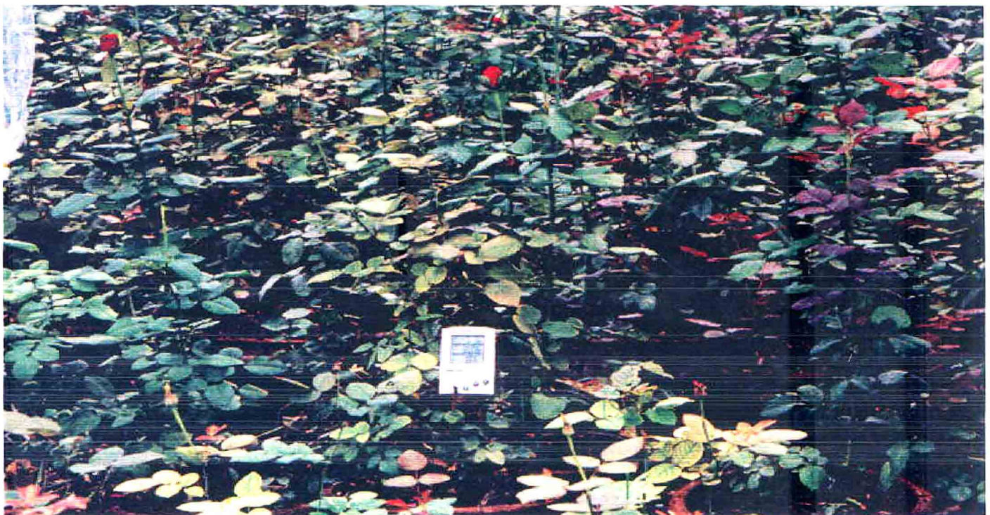
Thermohygrometer placed in crop canopy
