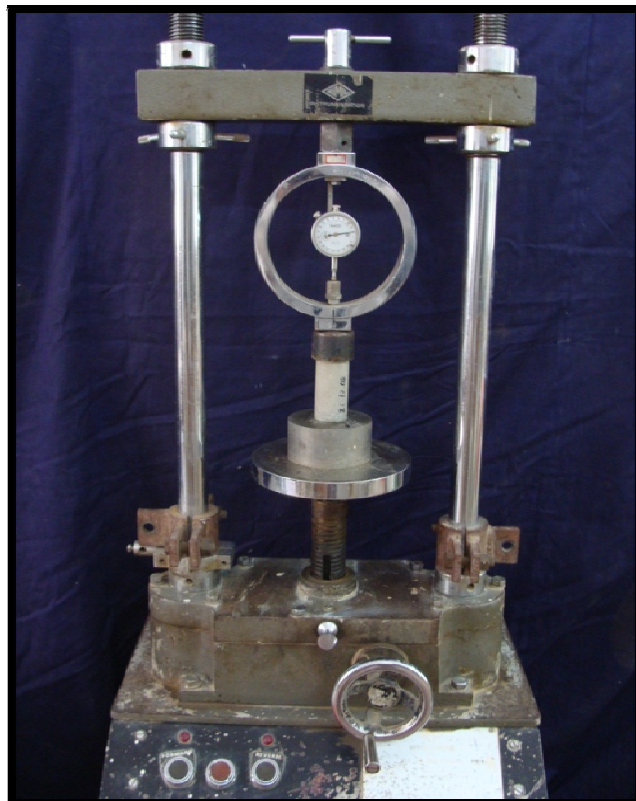
Plate 3.2 Compression tester for measurement of compressive strength
