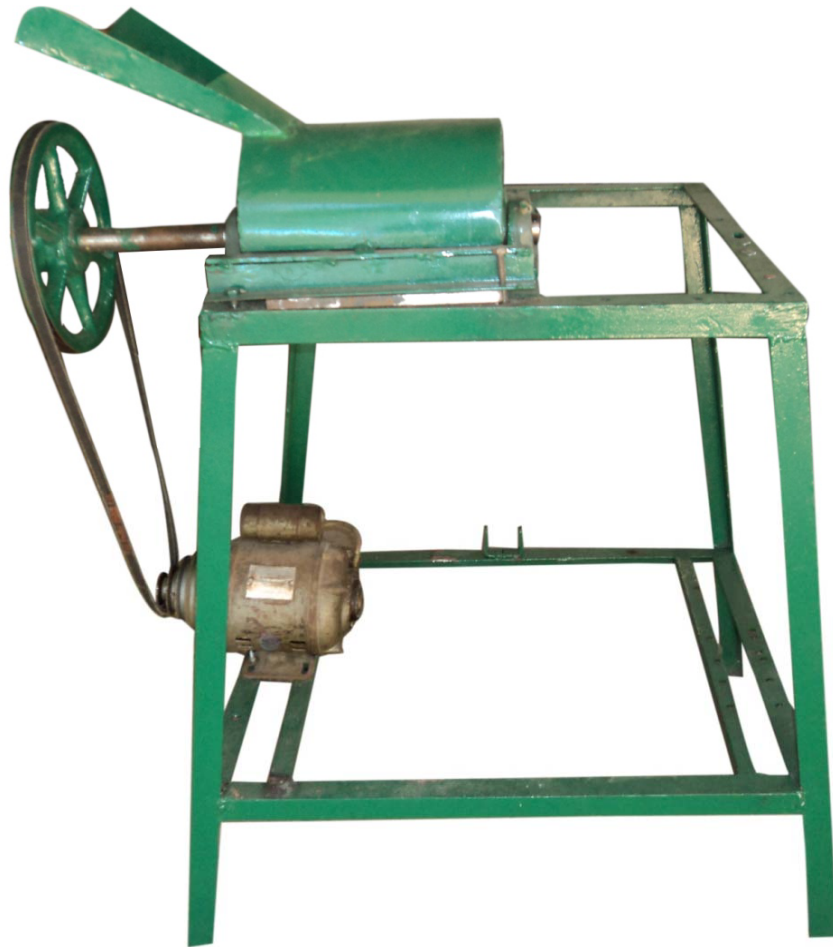
Plate 3.3 View of developed nutmeg decorticator and its cylinder
