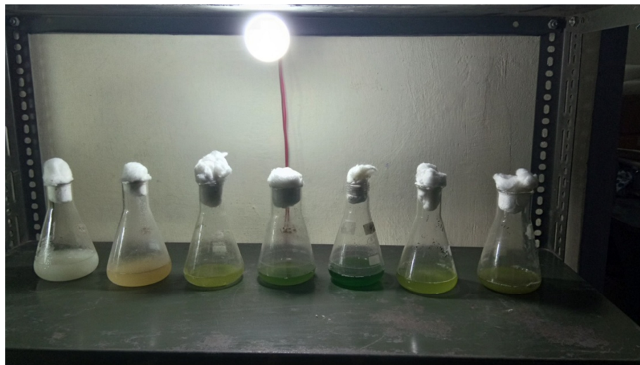
Plate VII a) and b) Microalgae grown on different concentrations of dairy wastewater under artificial LED light system, temperature =28\pm 2^{\circ}\text{C} at lab scale
