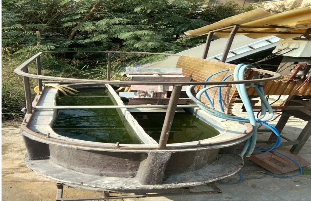
Plate V Mass cultivation of BGLRS BGLRS ( Scenedesmus sp. MKB.) in outdoor algal raceway pond
