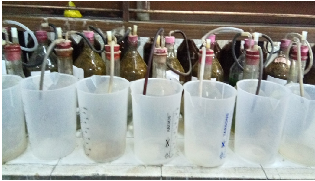
Plate III Biogas production from microalgae and paddy straw at lab scale
