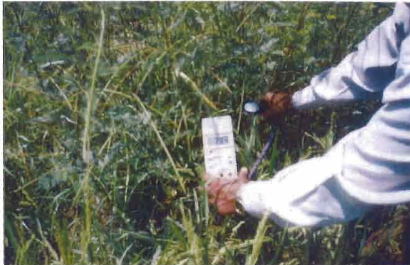
Plate :11 Recording - light availability (Canopy Bottom)
