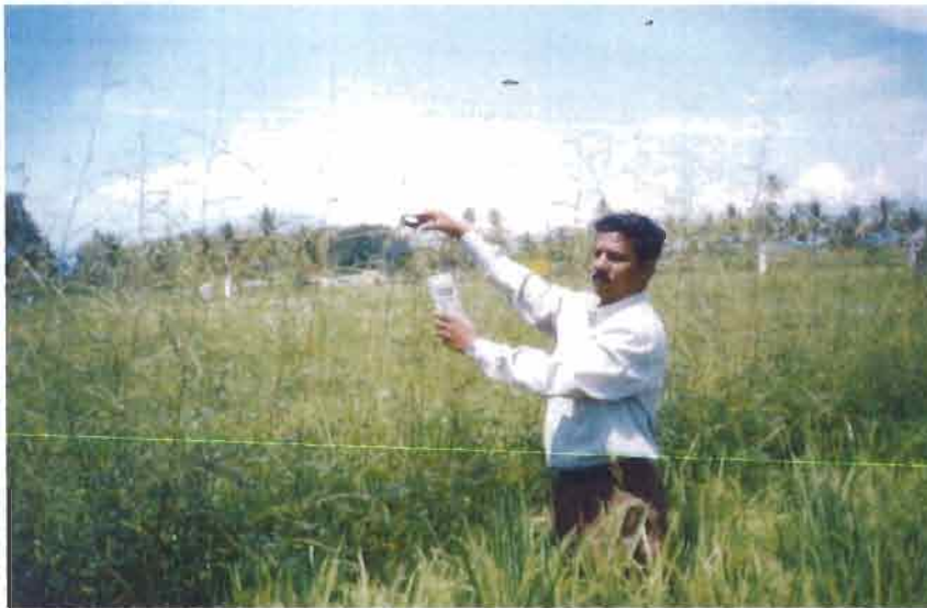
Plate :10 Recording - light availability (Canopy Top)
