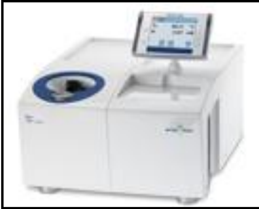
Differential scanning calorimetry (DSC) equipment for identifying gelatinization profile
