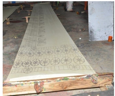
Figure 3.58. Fixing outline saree on to the maggam.
