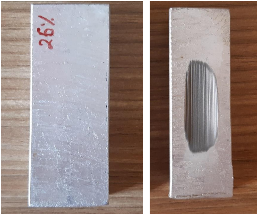
Figure 3.4(h): Sample before and after abrasion test
