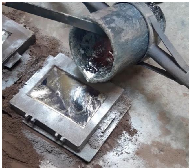
Figure 3.4(c) Pouring the molten metal and solidification
