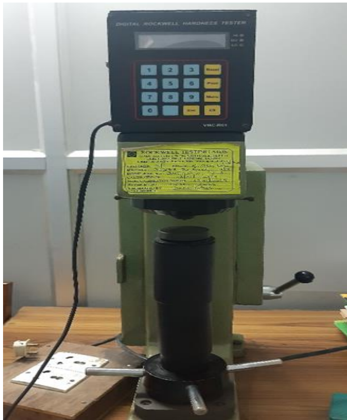
Figure 3.5(b) Rockwell Hardness Testing Machine
