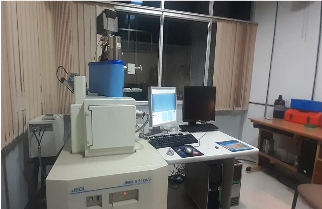
Figure 3.6(i): Scanning electron microscopy (SEM) setup
