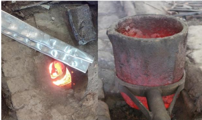
Figure 3.4(a) Melting of aluminium sheet and heated furnace
