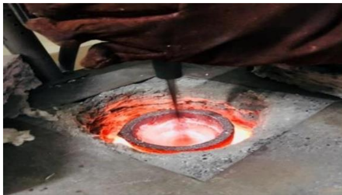
Figure 3.4(b) Stirring the mixture of Aluminium 1070 and SiC
