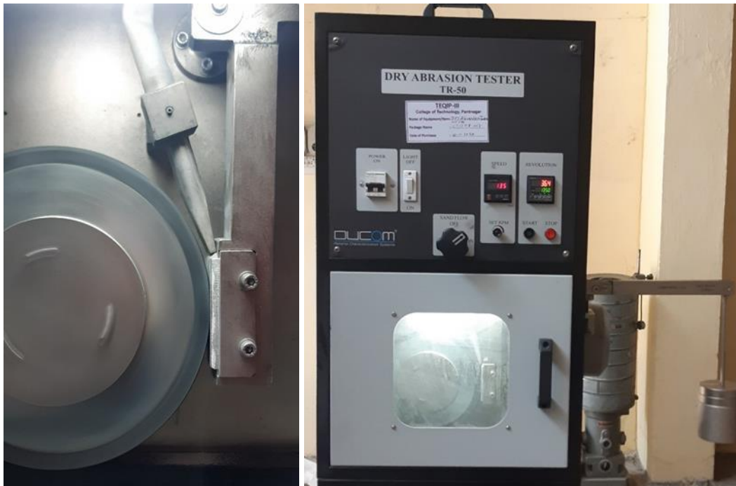
Figure 3.5(g): Dry sand abrasion test setup
