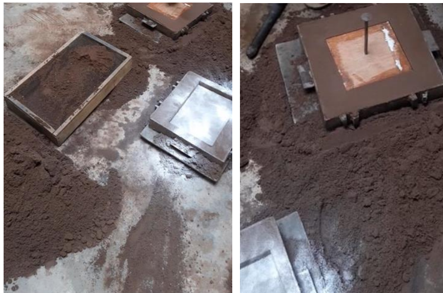
Figure 3.3(c) Preparation of sand and mould used in the cope and drag arrangement
