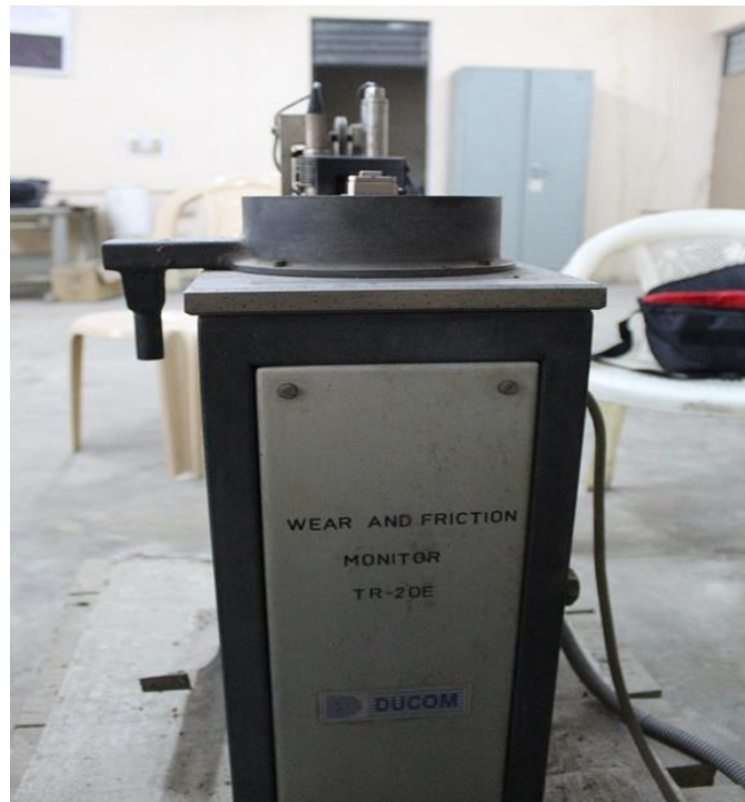
Figure 3.5(f): Pin on disc testing machine
