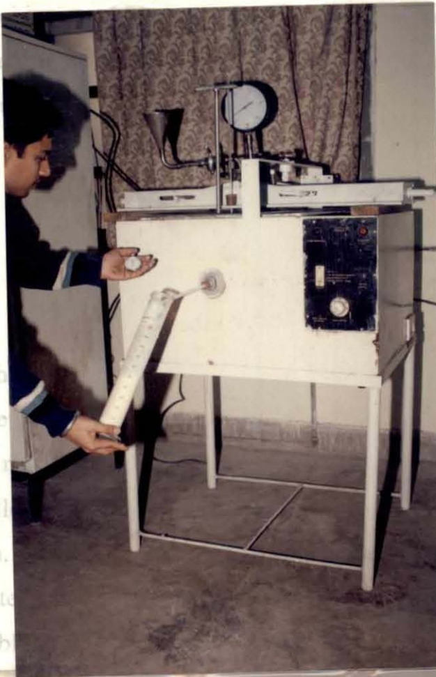
Plate-3: Constant temperature capillary tube viscometer in operation.
