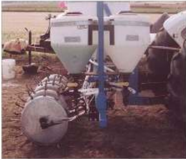
1. Handle 2. Fertilizer tank 3. Frame 4. Ground wheel 5. Skid 6. Furrow opener 7. Delivery tube 8. Furrow cleaner, a. PVC roller b. stainless-steel shaft c. semi-circular cover d. steel plate (Bautista and Schnier 1989)
