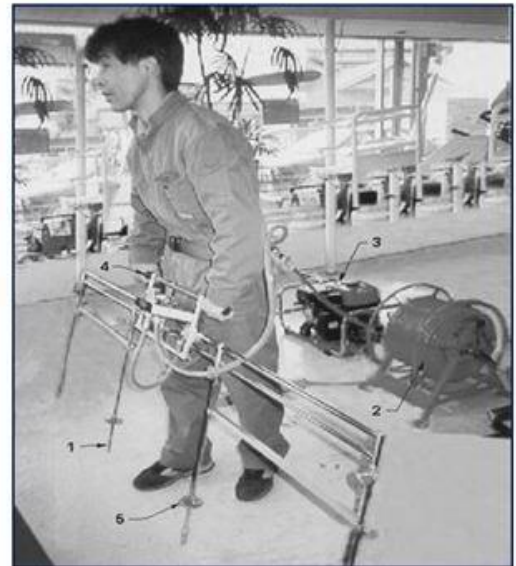
1. Injection nozzle 2. Connecting- hose 3. Engine-pump assembly 4. Handle 5. Depth-control plate (Hiraizumi 1997)
