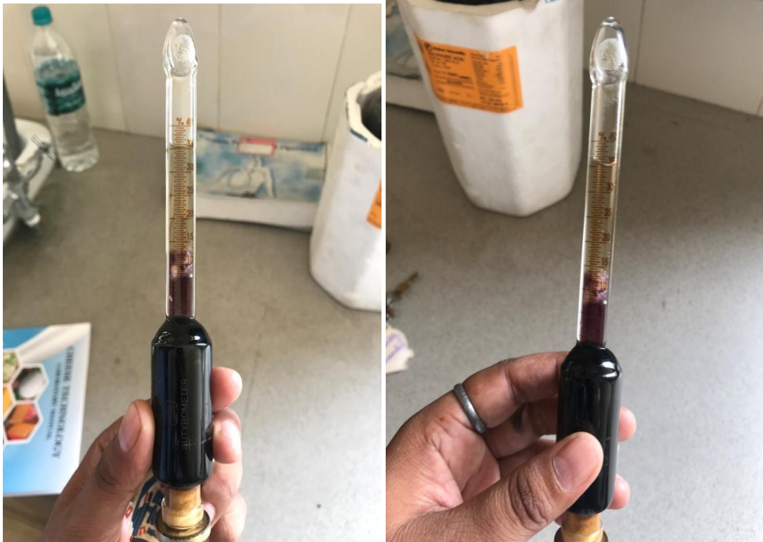
Fig. 3.19: Fat test of sample in cheese butyrometer
