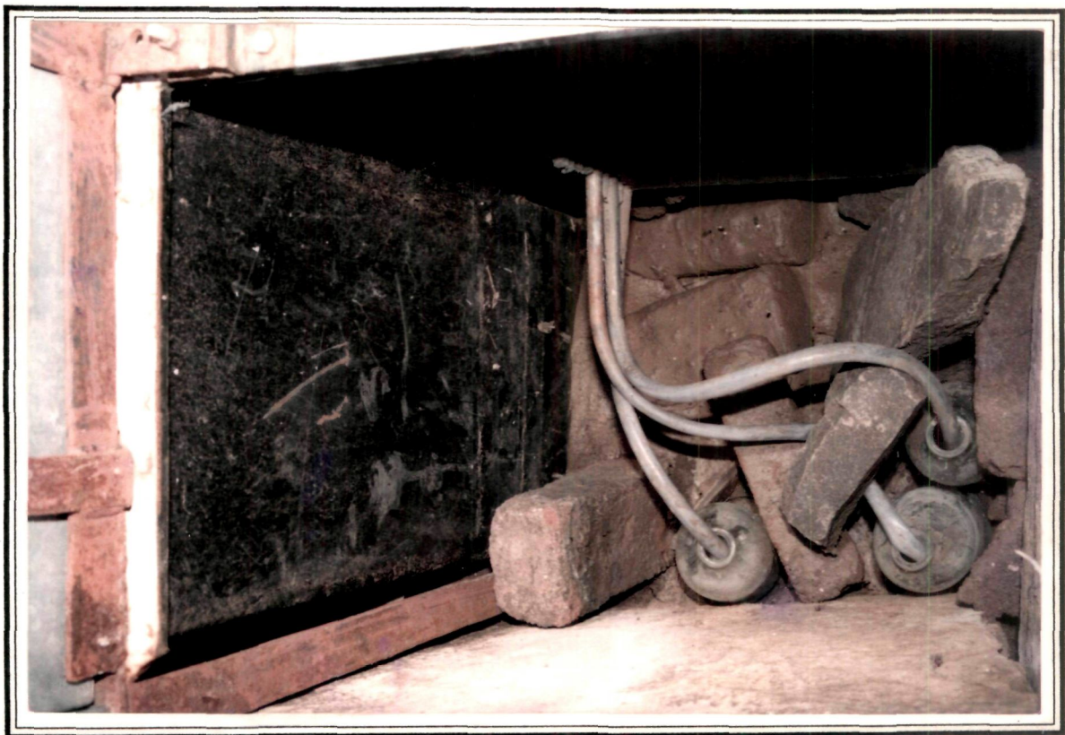
Plate 5. A top view of sediment samplers attached to the San Dimass flume to trap the portion of runoff
