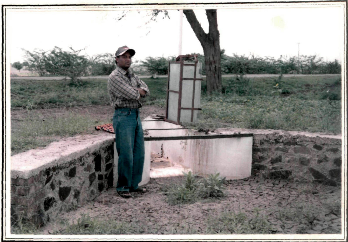
Plate 1. A view of experimental setup at the outlet including San Dimas flume and height level recorder
