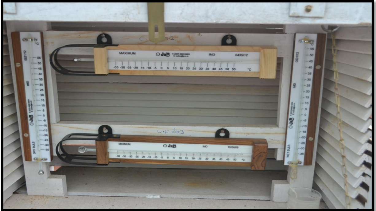
Plate 3.2 Stevenson's screen internal view
