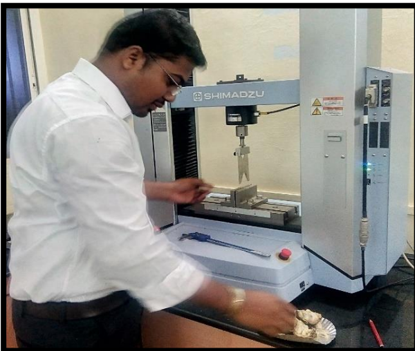
Plate 3.8 Measurement of Seed separation force
