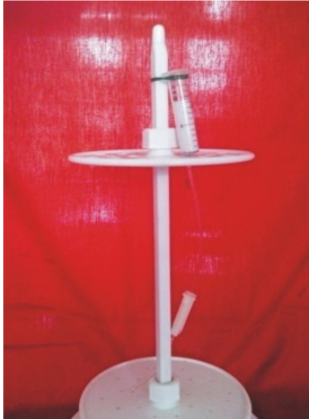
Plate 1. Cellulose column used for purification of IgG
