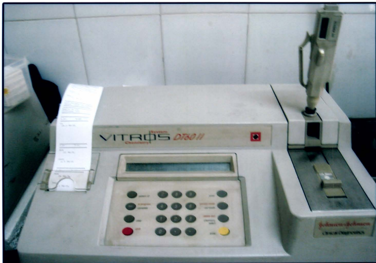
Plate 10. VITROS DT60 II chemistry system instrument, which was used for analysis of blood urea nitrogen and blood phosphorous.
