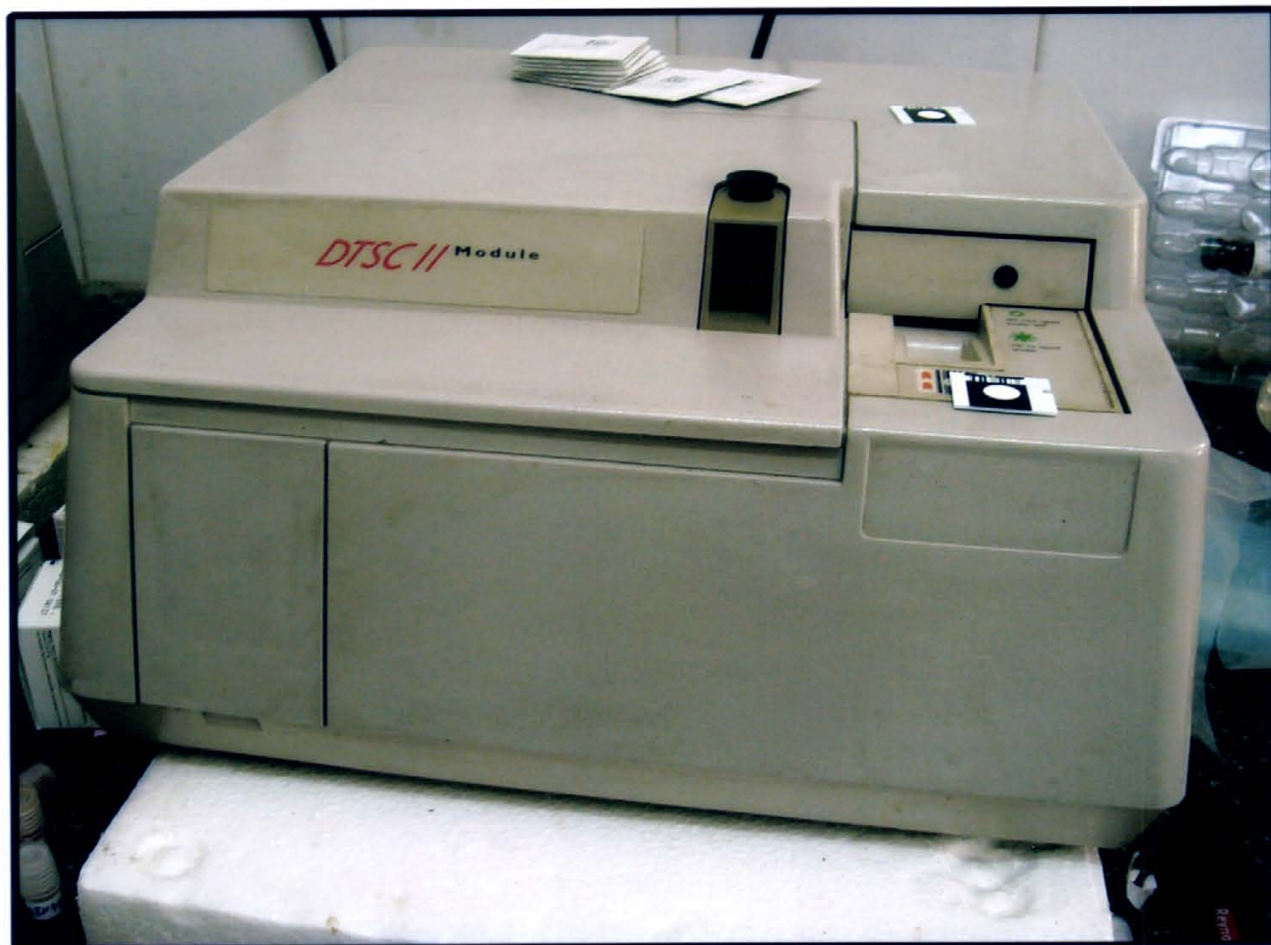
Plate 10. VITROS DT60 II chemistry system instrument, which was used for analysis of blood urea nitrogen and blood phosphorous.
