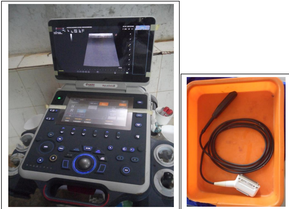
Plate 4.a. Esoate veterinary ultrasound scanner with SV 3513 probe
