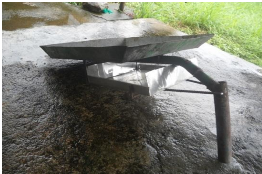
Plate 3.b. Removable tray of movable trevis for placing the scanner
