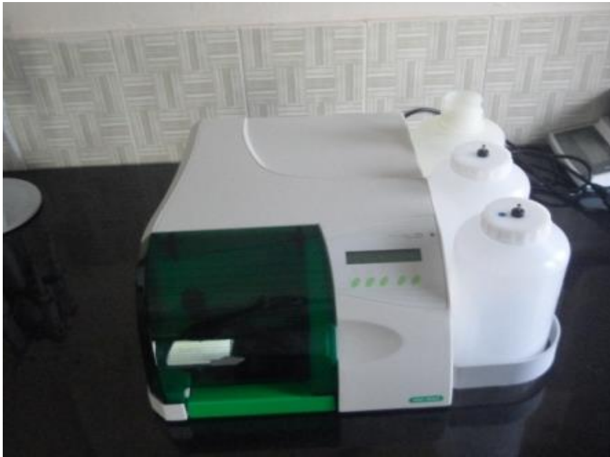
Plate 6.a. Bio Rad micro plate washer (Immuno wash Model 1575)
