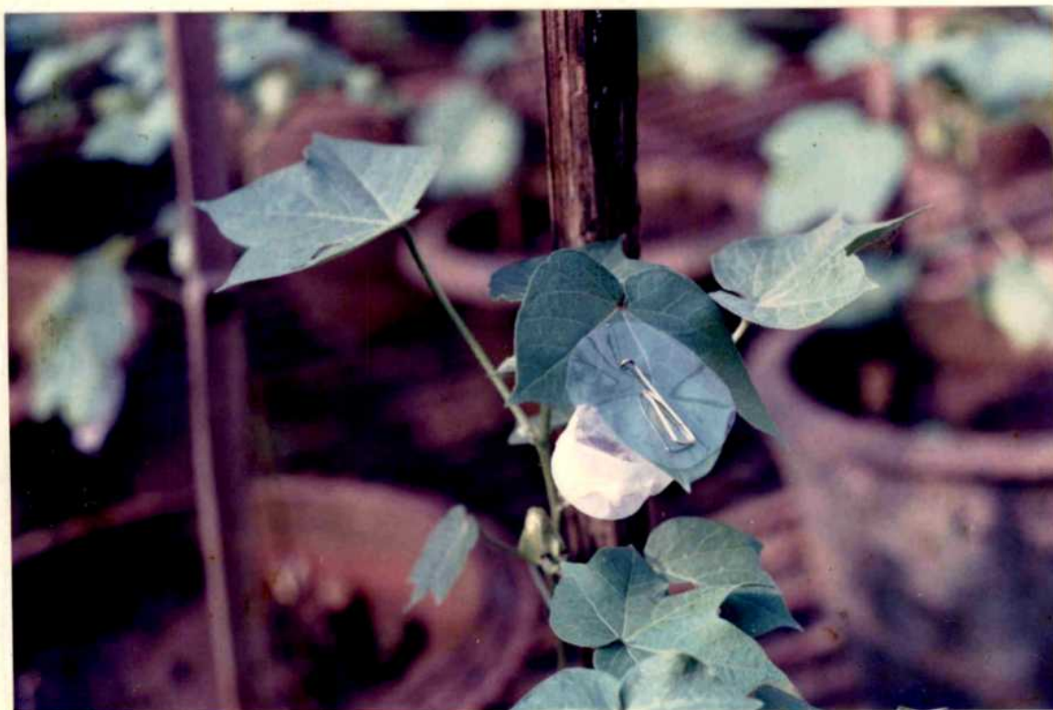
Plate 2. Microcage for persistent toxicity studies - Cotton
