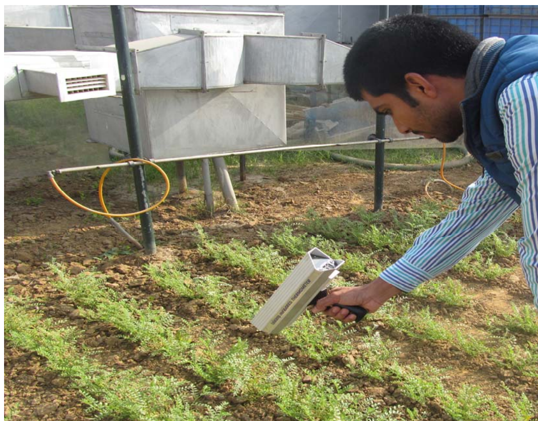
Plate 7. Measurement of canopy temperature using IR thermometer.
