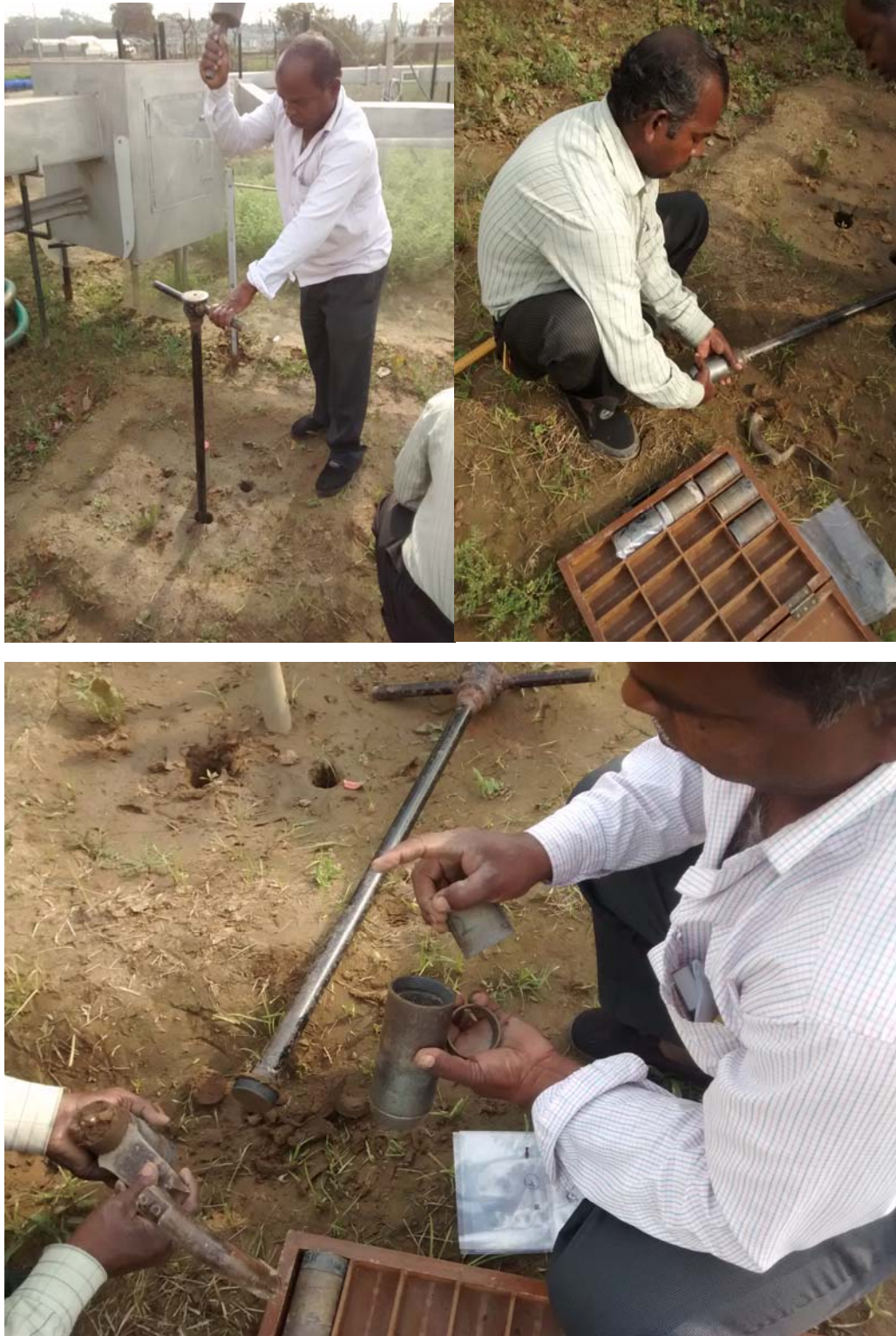
Plate 9. Bulk density measurement of soil profile for calibration of neutron moisture meter
