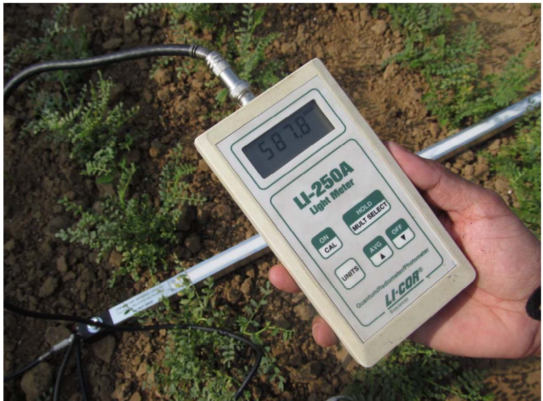
Plate 6. Measurement of PAR using line quantum sensor
