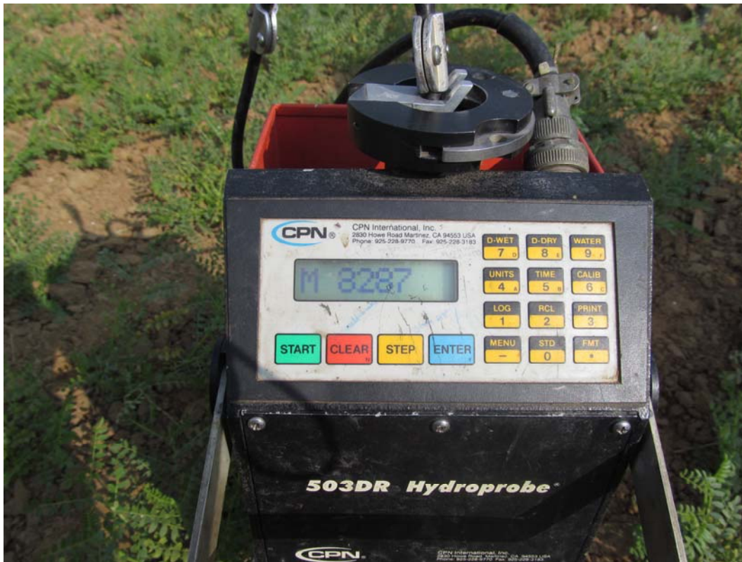
Plate 10. Measurement of profile soil moisture variation using neutron moisture meter
