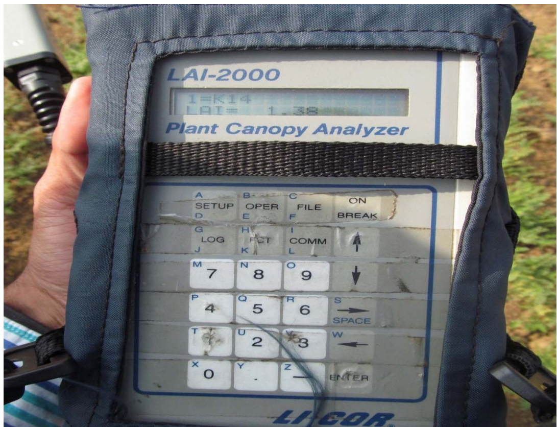
Plate 2. Measurement of Leaf Area Index using Canopy analyser
