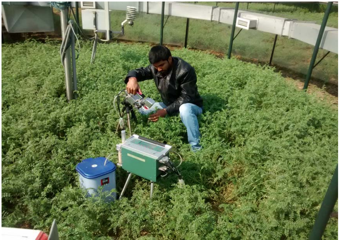
Plate 5. Measurement of photosynthesis and transpiration rate using IR gas analyser
