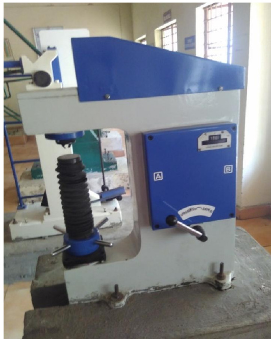
Plate 3.14: A view of Rockwell hardness tester
