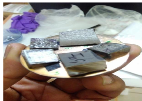
Plate 3.21: A view of sample holder for SEM
