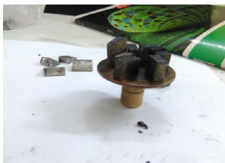
Plate 3.21: A view of sample holder for SEM
