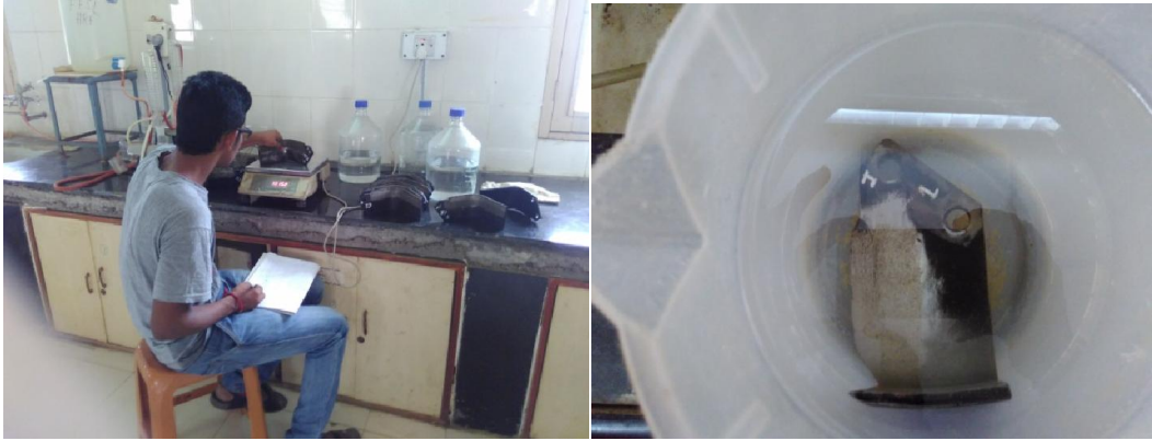
Plate 3.10: A view of measurement of weight and volume of blade
