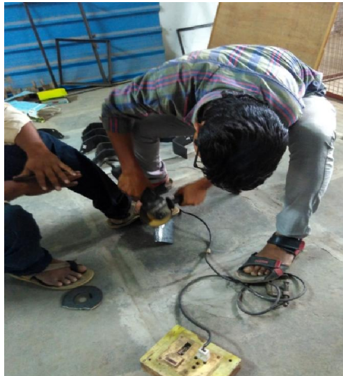
Plate 3.3: A view of polishing of coating surface of rotavator blade
