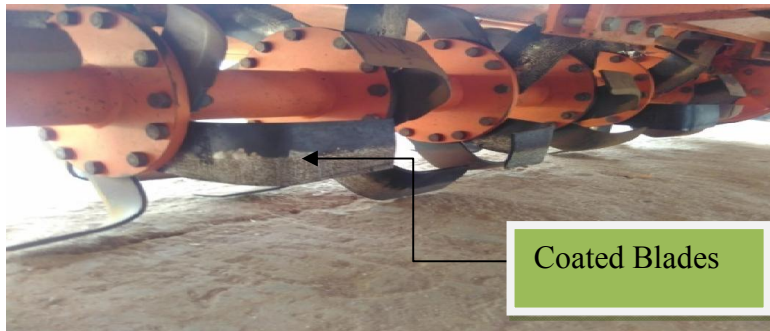
Plate 3.12: A view of rotavator after assembled of coated blades
