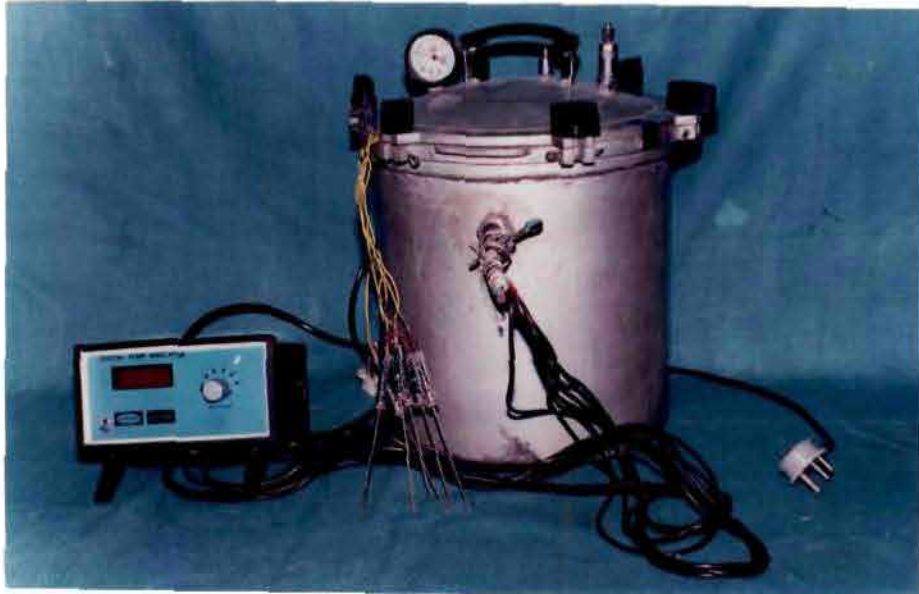
Plate 3: Fabricated laboratory type still retort with pressure gauge and six channel digital temperature indicator
