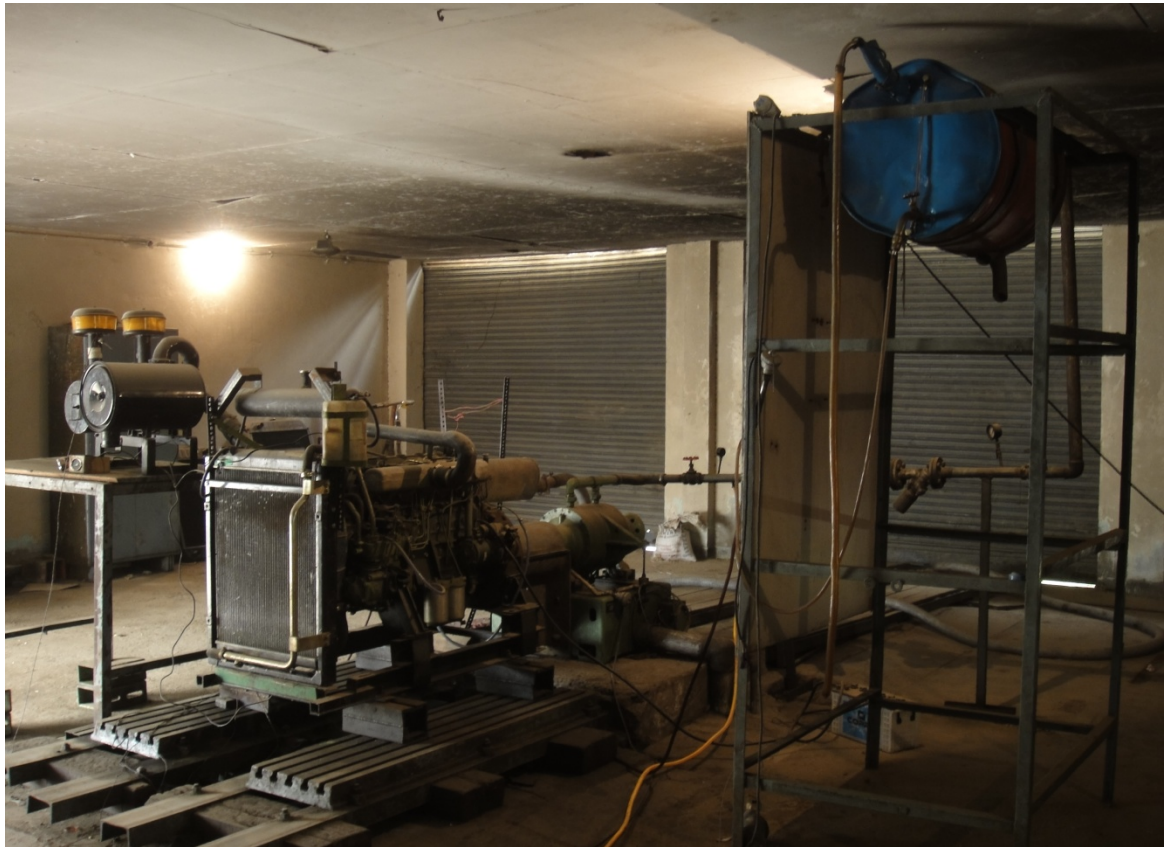
Plate: 3.2 Engine of combine mounted on testing-bed for testing
