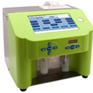
Fig. 3.5: Lactoscan milk composition analyzer
