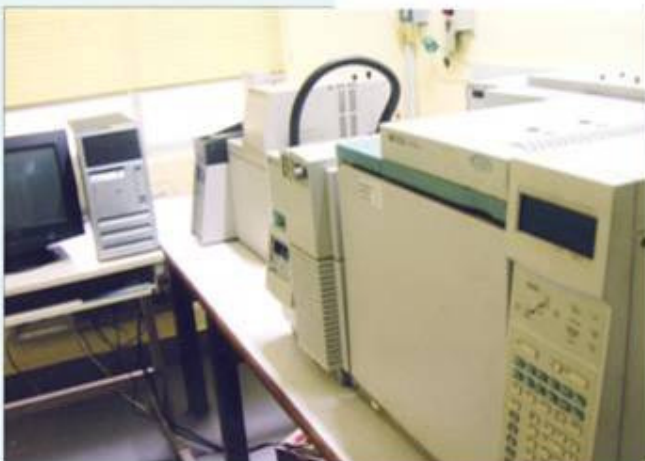
Plate 8. A view of GCMS setup used for identification of volatile compounds from cotton and sunflower
