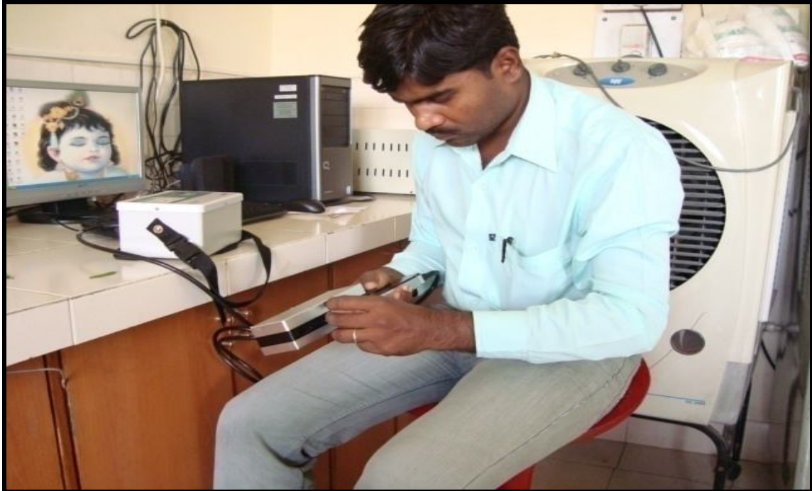
Plate 3.3 Leaf area measured through Leaf area meter
