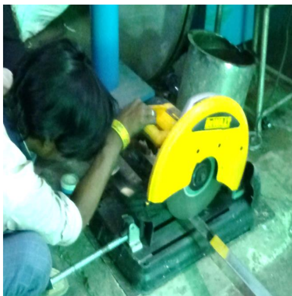
Cutting operation of square pipe
