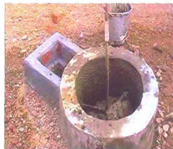
B. Gober gas production unit utilising the cowdung in a homegarden system – commonly seen in homegardens with livestock component
