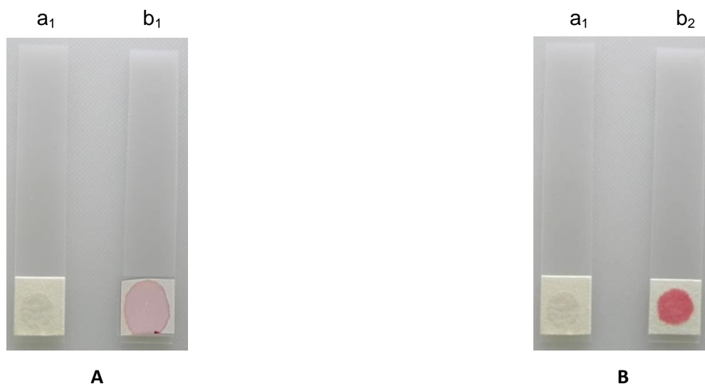
Figure 4.30. Detection of sucrose in khoa. (A). Detection of sucrose at 0.5% level; (B). Detection of sucrose at 1% level (a 1 - pure khoa , b 1 - khoa prepared from milk containing 0.5% sucrose, b 2 - khoa prepared from milk containing 1% glucose)
