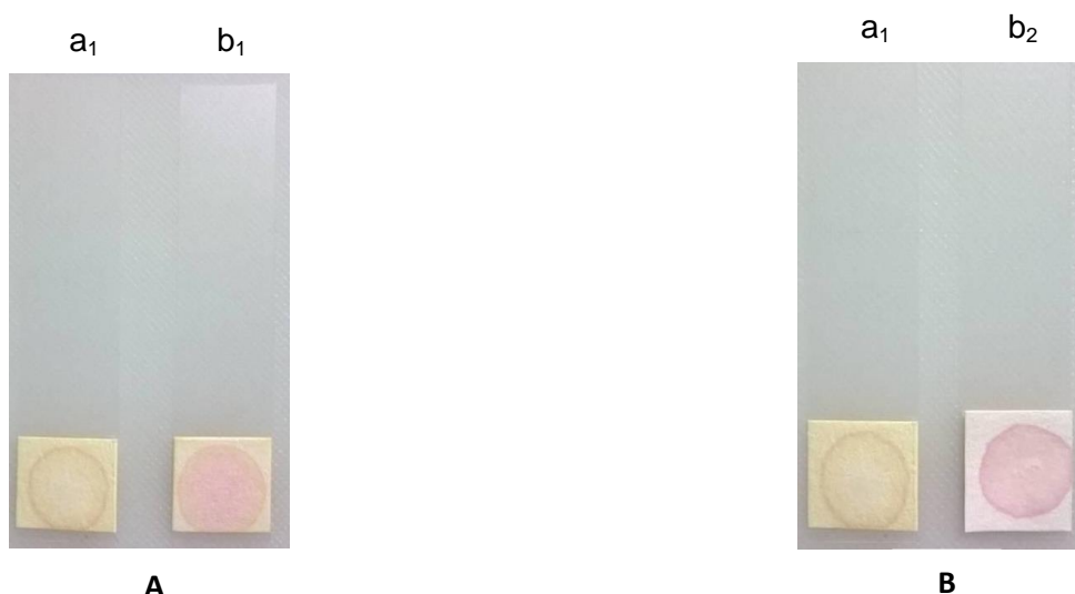
Figure 4.33 Detection of sucrose in Dahi . (A). Detection of sucrose at 0.5% level; (B). Detection of sucrose at 1% level (a 1 - pure Dahi , b 1 - Dahi prepared from milk containing 0.5% sucrose, b 2 - Dahi prepared from milk containing 1% sucrose)
