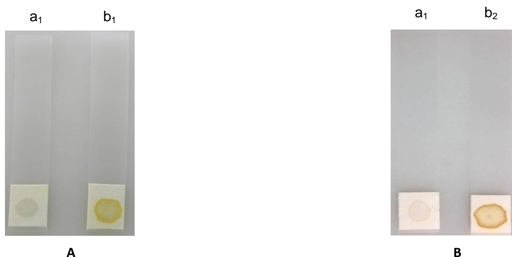
Figure 4.31 Detection of maltodextrin in khoa. (A). Detection of maltodextrin at 0.5% level; (B). Detection of maltodextrin at 1% level (a 1 - pure khoa , b 1 - khoa prepared from milk containing 0.5% maltodextrin, b 2 - khoa prepared from milk containing 1% maltodextrin)
