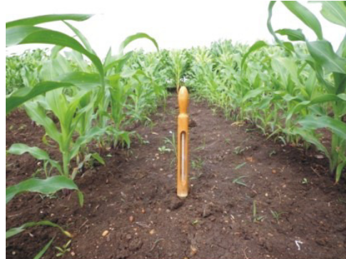
Soil temperature observation using soil thermometer
