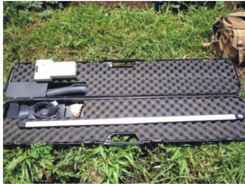
Line quantum sensor with data logger
