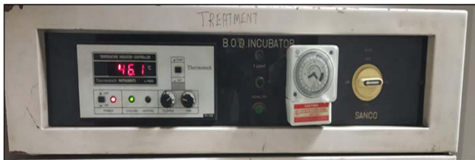
Plate 2. Incubator with temperature controlling facility for maintaining required temperatures for thermal stress
